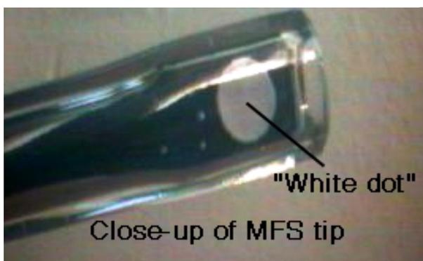
**Fig. 2** A close-up of the MFS tip. The actual sensor is the "White dot".
