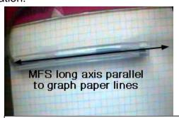
**Fig. 1** Place the MFS sensor tube so that it is parallel to the graph paper lines. Tape it (and the graph paper) down so that things stay put for the duration of the experiment.
