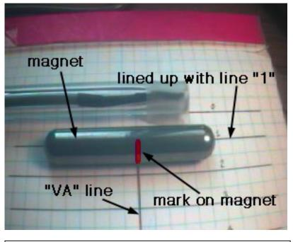
**Fig. 5** Placing the magnet on the page. Place the magnet along line "1", parallel to the line. Draw a "VA" (visual-aid) line as shown in the picture. Make a small mark on the magnet, using a permanent marker, where the magnet intersects the VA line.
